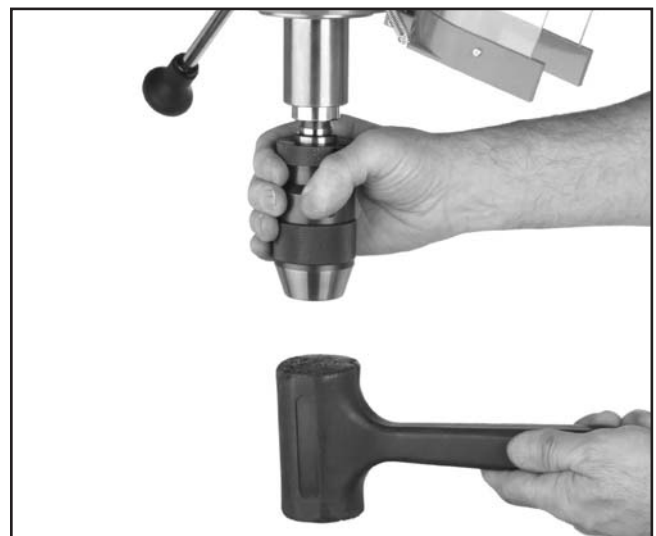
Figure 17. Seating arbor and chuck into spindle.
